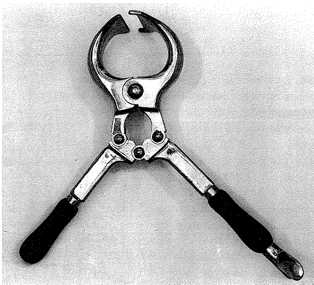
Fig. 4.2. The Burdizzo. Note that one jaw of the Burdizzo is extended laterally so that it overlaps at each end (the cord stop). This is to prevent the spermatic cord slipping from between the jaws when they are closed.
