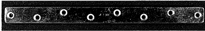
Fig. 10.205. Heavy duty bone plate. This plate is 4.8 mm thick and obtainable with either screw holes or slots to the following lengths: 150 mm, 180 mm and 205 mm. It is drilled and countersunk to accept 4-mm bone screws. This plate is useful for the fixation of fractures in large dogs.
