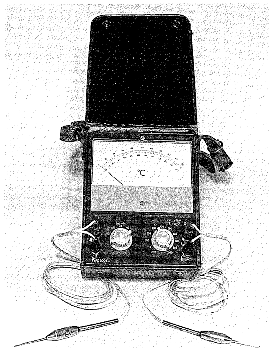
Fig. 12.16. Tissue temperature monitoring device together with tissue probes.
