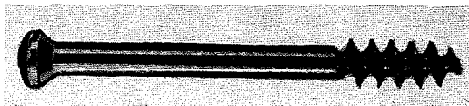
Fig. 10.1. 6.5-mm cancellous bone screw. Diameter of thread 6.5 mm; diameter of core 3.2 mm; diameter of shaft 4.5 mm.
