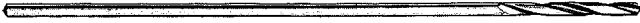
Fig. 10.217. Drills. Bone drills are made from either stainless steel or vitallium. Stainless steel twist drills are obtained in the following sizes:
